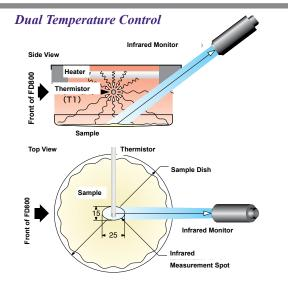
In addition to the ambient temperature in the drying chamber (T1), the FD800 monitors sample temperature (T2) <sup>(Patent pending)</sup>, providing unsurpassed drying control, resulting in optimized drying times, and minimizing or eliminating sample degradation and resulting measurement accuracy.
