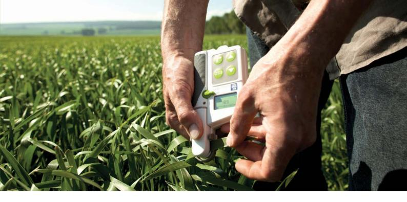
For this approach, rather than taking the typical 'W' pattern through a field, a small, repeatable area that is representative should be chosen to take the 30 samples. Also, rather than selecting the crop in the options on the screen, scroll down and select '(with reference)'. A field name can then be entered, after which the samples can be taken, ensuring the youngest fully emerged leaf is chosen each time.
