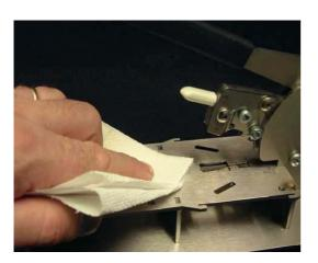
Remove the shim plate and wipe it clean. Note the shim plate is not stainless and some additives in certain oils may cause staining ( this is not a functional problem).
