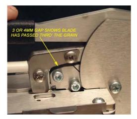
With maize being such a hard grain, a significant increase of effort at the operating lever will be required to initiate the second phase. Once started, phase two occurs with little effort as the knife passes right through the clamped grain. The handle then experiences distinct resistance as the "tooth" cam engages with the shutters.
