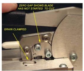
When the operating lever is pulled down there are three distinct phases to the cutting cycle which can be felt. The first resistance is felt when the "V" clamp aligns and locks the grain. At this point the knife has still not yet started cutting the grain.
