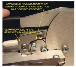
Further pressure on the operating lever opens the shutters and allows the sprung loaded "V" clamp to pass through the shutters, this clamp then becomes an ejector to send the split grain into the two collecting trays.
