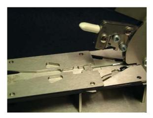
Slide the top plate off and wipe any oil from the underside
