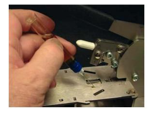
The bed plate around the shutter area should be oiled with a THIN film of oil -5 or 6 drops of oil smeared around with a finger tip) and
